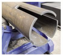
Area for cutting pipes, square and rectangular profiles equipped with rotary pipe positioner
