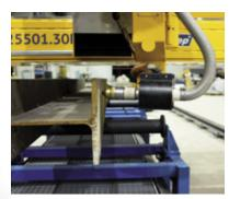
Cutting of structural profiles as I,H,U and L in separate area
